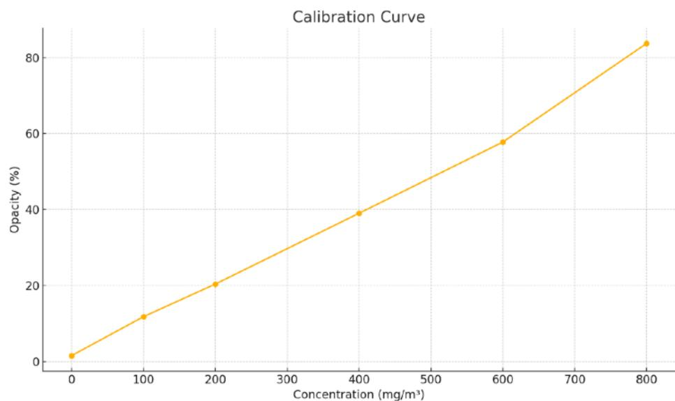
Demonstrates the analyzer's linear response (opacity vs. concentration) and its high-accuracy span calibration.
