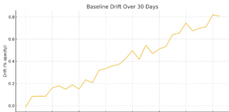
Illustrates the device's long-term stability (drift <1% opacity/month) and the need for occasional calibration checks.
